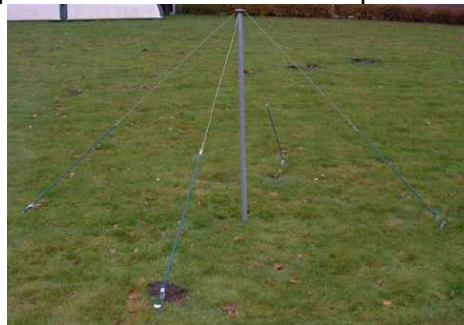
FIGURE 2. The Low Frequency Antenna used in the Cosmic Rays Radio Detector experiment.
